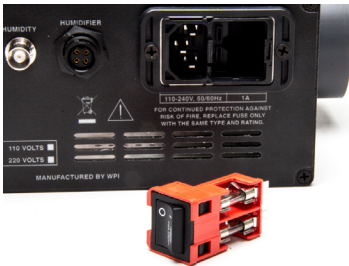
Fig. 29—Remove the fuse housing to access the fuses.
