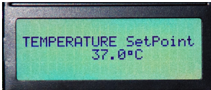
Fig. 6—Press TEMP to display the temperature setpoint.
