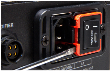
Fig. 27—(Left) Insert the screw driver under the fuse housing lip and pry the housing open.
